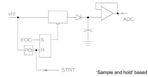
Once the conversion is completed the ADC contents are transferred to memory register and memory contents of the location at the address are incremented by one, indicating the even (pulse) with height in the interval.
