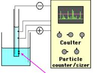
When particle passes through the gap between two electrodes, the resistance of the changes is detected and converted into a pulse (signal) the height of which provides information regarding particle size.
