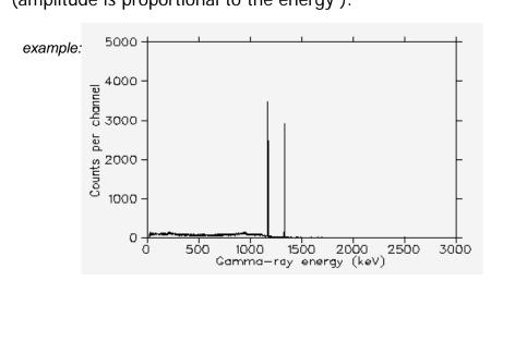
Sorting by height is equivalent to sorting by energy (amplitude is proportional to the energy ).
