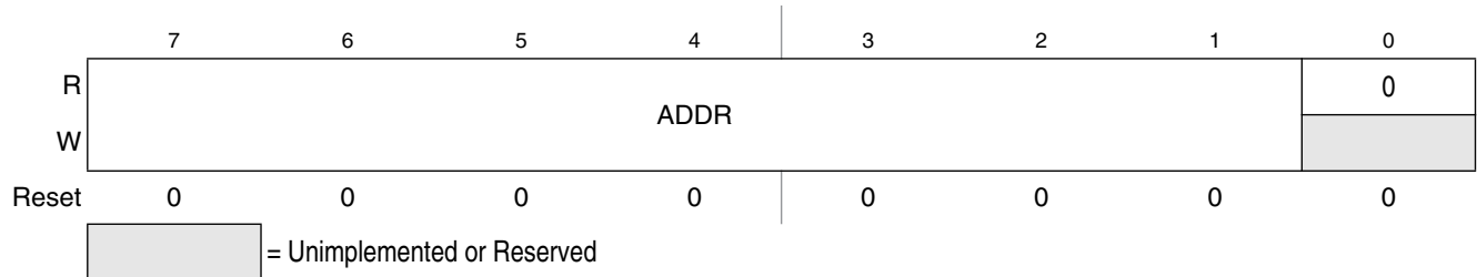
Figure 11-5. IIC Address Register (IICA)
