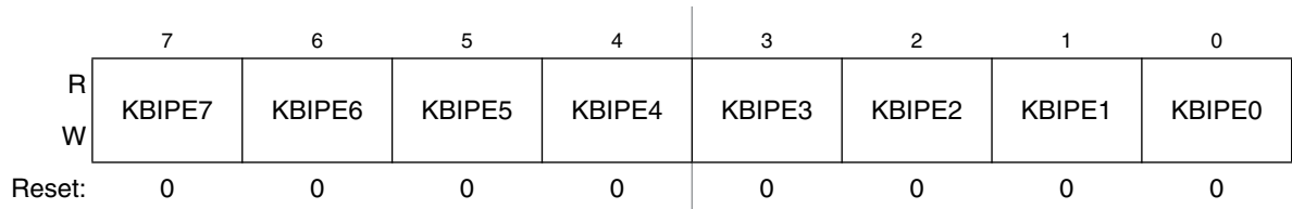
Figure 12-4. KBI Pin Enable Register
