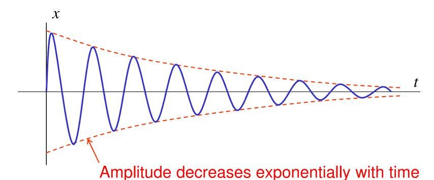
Without damping: the angular frequency is  $\omega_0 = \sqrt{\frac{k}{m}}$
