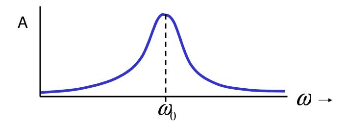
Resonance occurs because the driving force changes direction at just the same rate as the "natural" oscillation would reverse direction, so the driving force reinforces the natural oscillation on every cycle.
