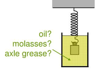
$b > 2m\omega_0$ : "Overdamped", no oscillation.
