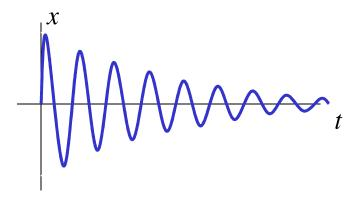
Damped Oscillator: Drag force  $\mathbf{f} = -b\mathbf{v}$
